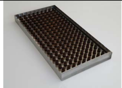
Full vial tray with vial positioner insert
